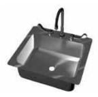
Stainless Steel Sink and Faucet Kit Includes 14" x 18" x 7<sup>1</sup>/<sub>2</sub>" (356 x 457 x 191mm) stainless steel sink bowl, chrome-plated faucet (6" [152mm] swivel gooseneck wrist blade handles) trap and drain.
